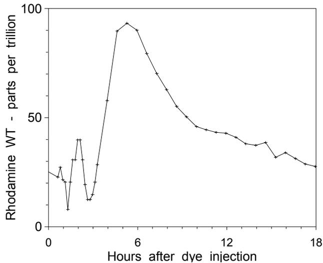
**Figure 1.** Breakthrough curve of a Rhodamine WT tracer test in dolomite from a borehole to a spring. Typical features shown are the rapid rise and exponential recession, and high sensitivity of the technique.
